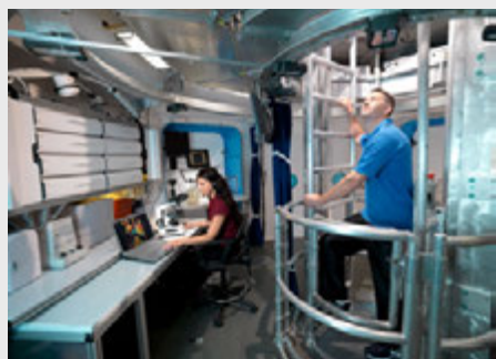
NASA's Human Exploration Research Analogue is used several times per year to understand and test mitigation strategies for human performance risks.
