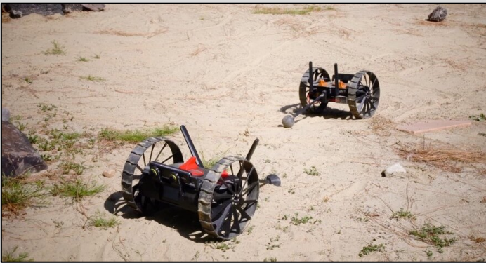
Multi-robot autonomy and commanding for distributed measurements (JPL, 2021) TRL 5
