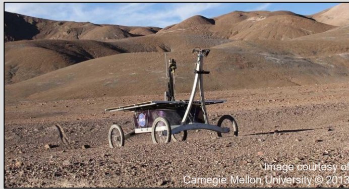
Autonomous rover traverse (26 km in 10 days) across the Atacama (CMU, 2015) TRL 5
