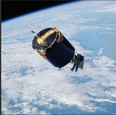
1984 – STS-51-A mission retrieves and de-orbits the defunct Westar 6 satellite after failed deployment
