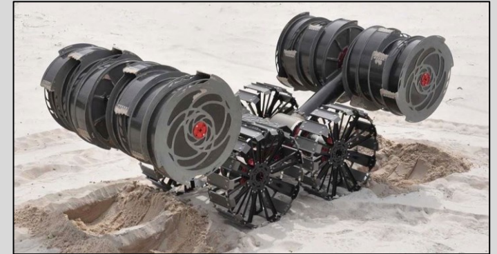
Prototype robot for excavation of lunar regolith (RASSOR, KSC, 2021) TRL 5
