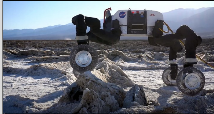
Traversing obstacles with 3x wheel radius with RoboSimian (JPL, 2020) TRL 5
