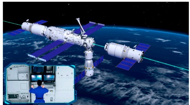
Fig. 26. The astronaut's remote control TZ-2 docking with TG.
