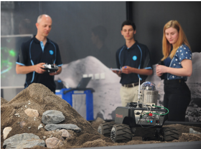
CSIRO ISRU team demonstrating its autonomous rover capabilities in a sealed lunar dust testbed environment with an intern student to inspire the next generation of space researchers. © CSIRO
