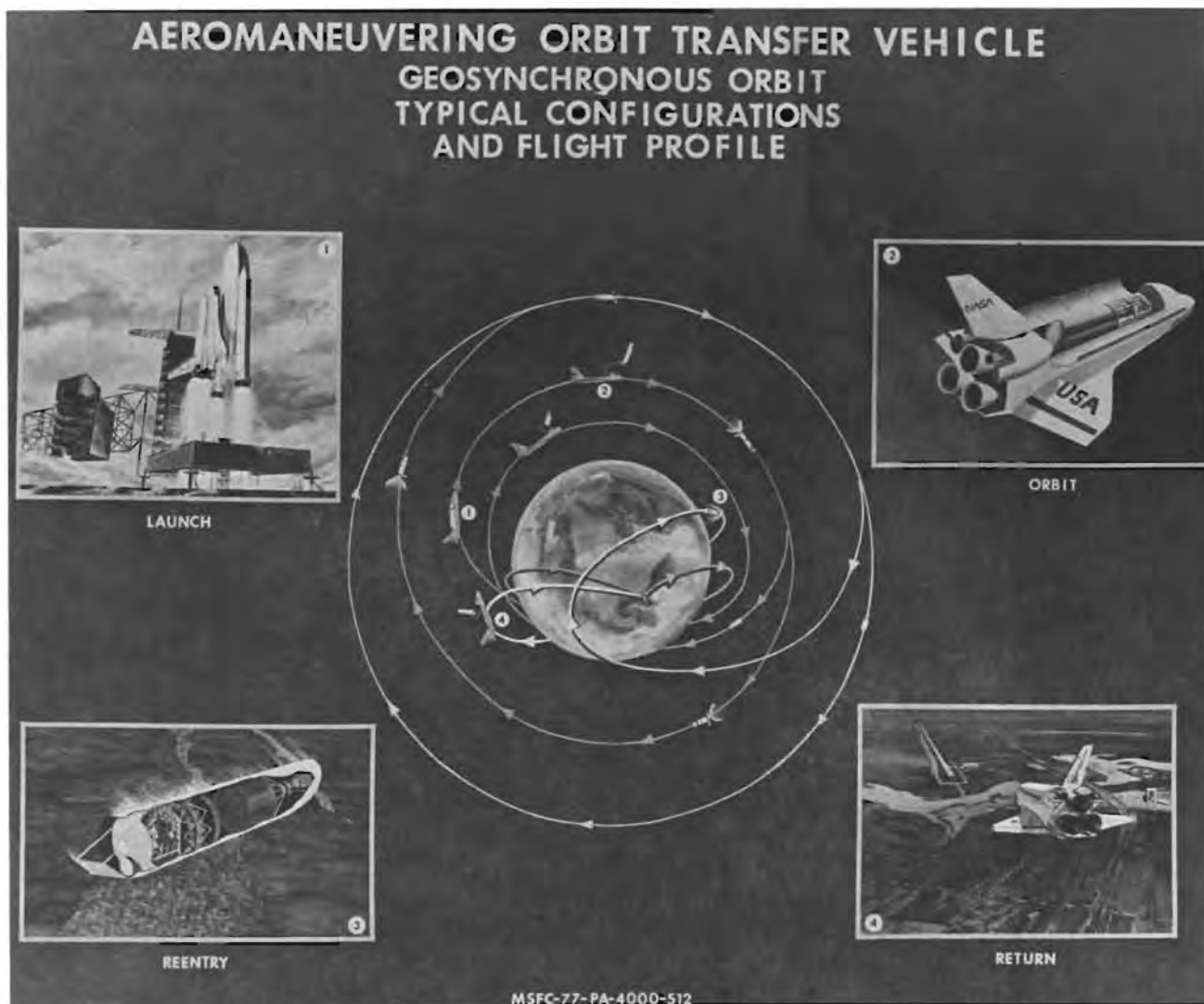
Figure 77. Aeromaneuvering orbit transfer vehicle geosynchronous orbit typical configurations and flight profile.
