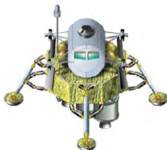
Layout of Solid Propulsion LSAM Descent Stage
