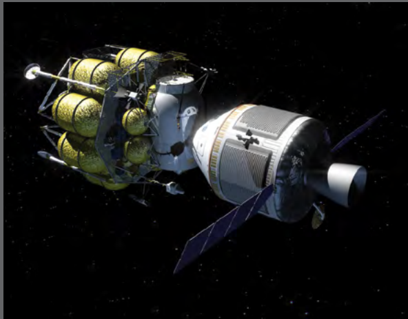
Crew Exploration Vehicle and NASA Lunar Surface Access Module, late 2005.
