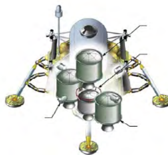
Layout of Solid Propulsion LSAM Ascent Stage
