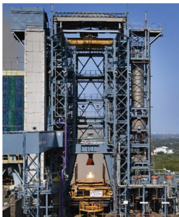
L110 Vikas engine hot test
