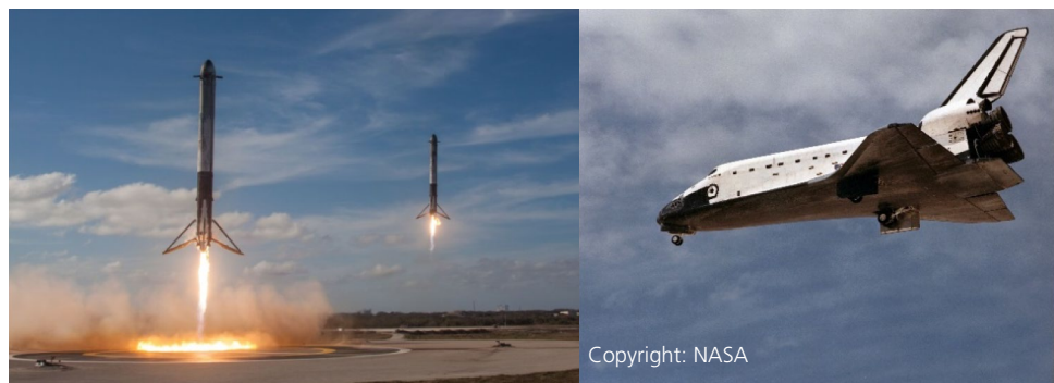
Fig. 1 Two prominent reusable launch stages: the Falcon heavy side boosters landing vertically, [2], and the Space Shuttle orbiter during the final approach landing horizontally, [3]
